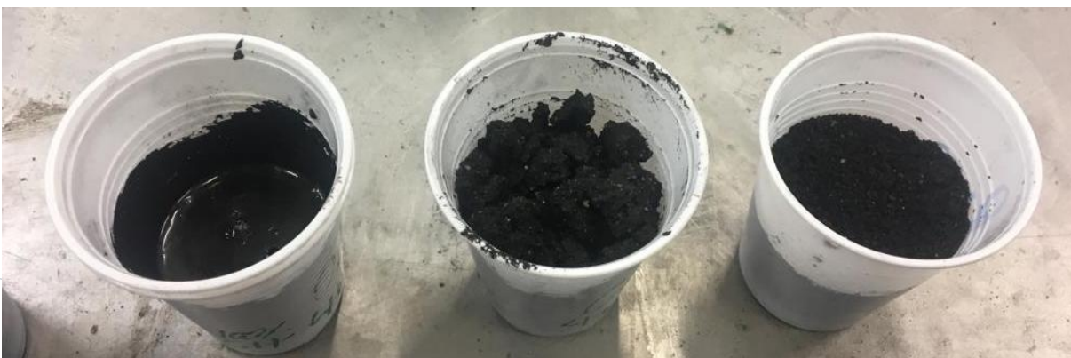
Figure 5. Different solution and same liquid to solid ratio. From left to right: Sodium Hydroxide only; Sodium Silicate and Sodium Silicate; and Sodium Silicate only.
