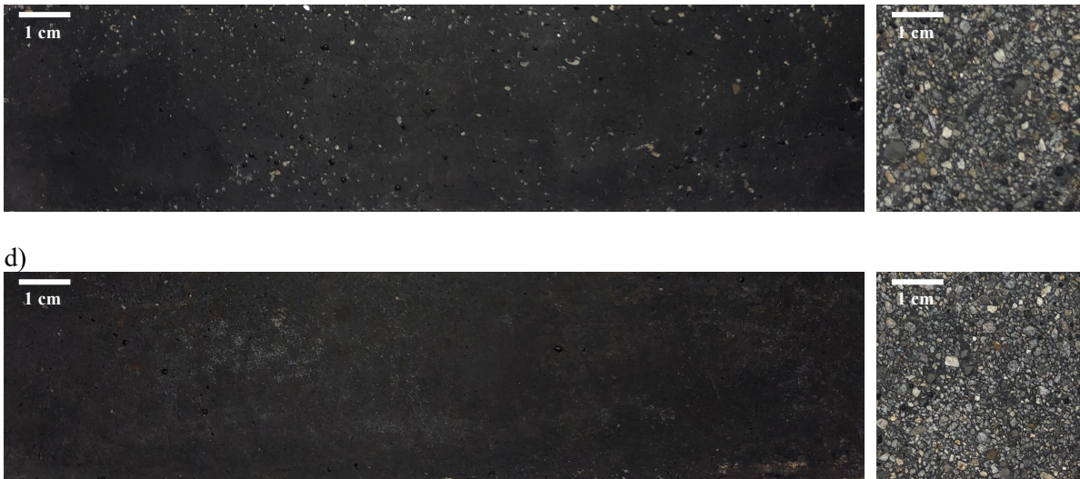
Figure 14. Surface and cross section of 50SSA50GBFS (a) 4M; (b) 6M; (c) 8M; and (d) 10M.
