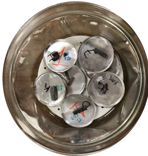
Figure 10. Set of samples drying for MIP testing.
